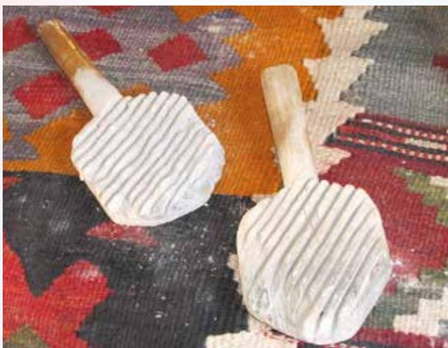
There is no need to dig deep pits for the ovens prepared by craftsmen. They spread the clay in a certain width and thickness, stacked around the circle, and fold up into pieces. At the same time, the craftsman keeps the clay with one hand and with the second hand beats the clay with a special wooden instrument so that the joints were unnoticeable and solid. Depending on the natural conditions, the oven is drained for 2–3 days and after it is installed and used.
